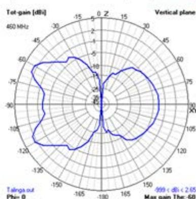
Figure 5: Simulated Antenna Pattern distortion at 1m from the tower
