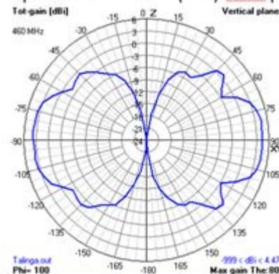
Figure 6: Simulated Antenna Pattern distortion at 2m from the steel tower
