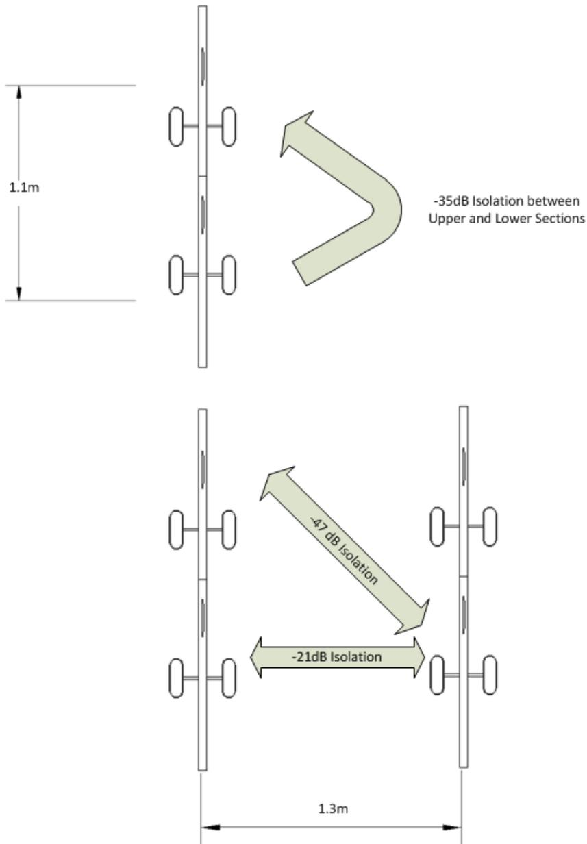
Figure 7: Antenna Isolation for dual stacked antenna configurations [5]
