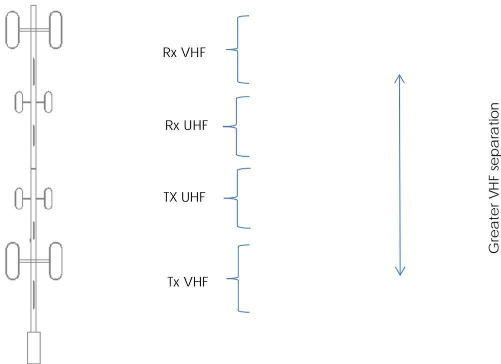
Figure 8: Dual band VHF and UHF stacked antenna configuration
