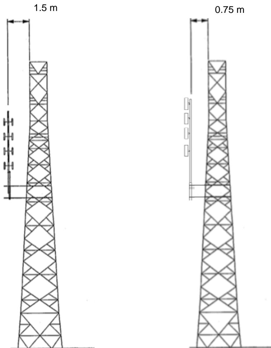
Figure 7: Tower separation for omni array and Directional array
